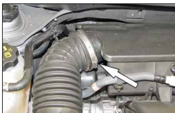
4. Loosen the hose clamp that secures the intake tube to the intake plenum.
