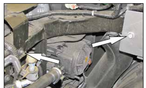
6. Remove the two factory bolts shown. NOTE: These bolts will be reused in a later step.
