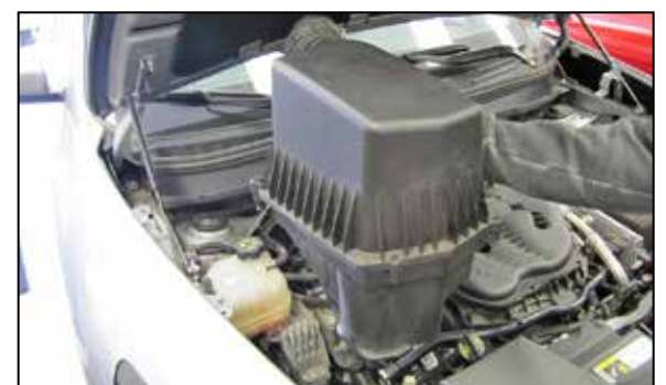
5. Lift up the air filter housing to dislodge it from the mounting grommets and then remove the complete air filter housing assembly from the vehicle. NOTE: K&N Engineering, Inc., recommends that customers do not discard factory air intake.
